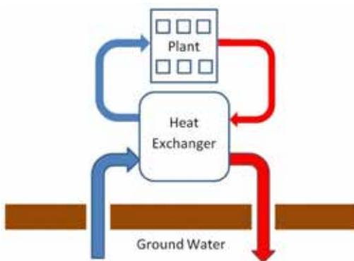
Schematic of a typical ground water cooling system
