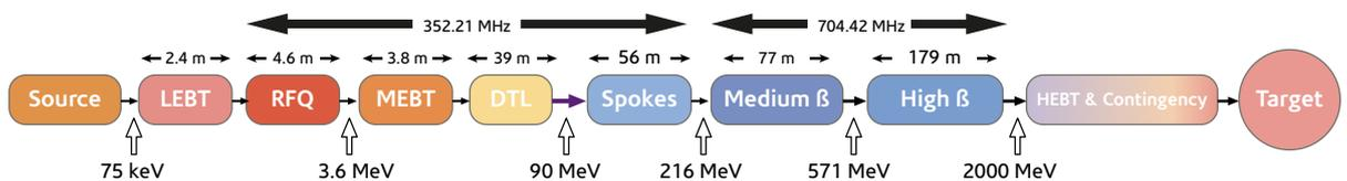
ESS Linac Layout (Courtesy: ESS)
