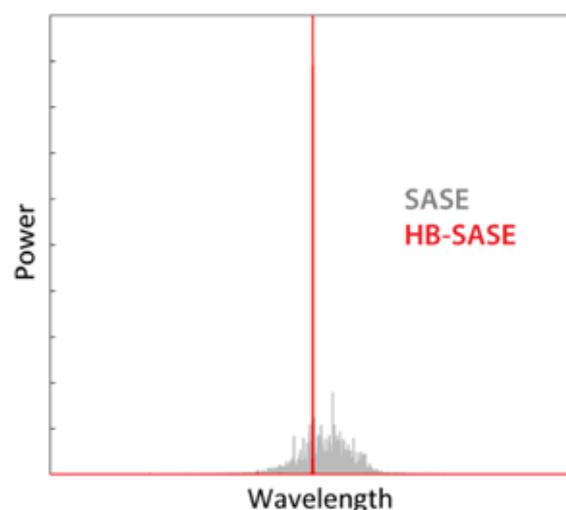
A comparison of FEL spectra for SASE and HB-SASE where the HB-SASE spectrum is effectively a single line, indicating a close to transform-limited pulse with full temporal coherence
