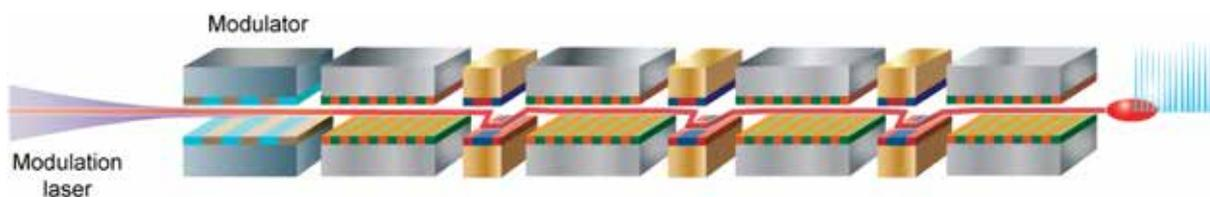
Schematic layout of a Mode-Locked FEL where a laser is used to add a periodic energy modulation to the electron bunch and decay chicanes are inserted periodically along the length of the undulator
