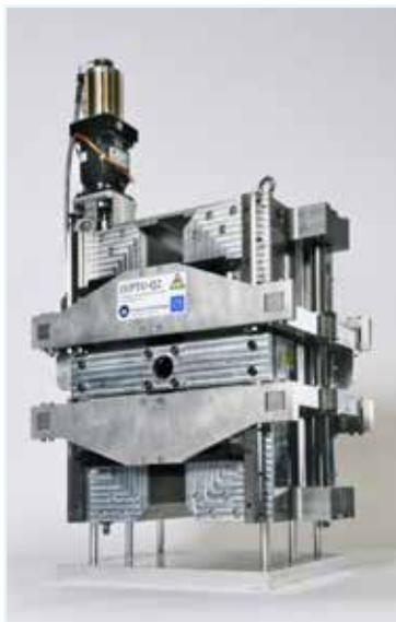
High-strength prototype quadrupole ZEPTO-Q1 and low-strength prototype quadrupole ZEPTO-Q2
