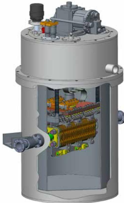
CAD model of the superconducting undulator prototype inside the cryostat.
