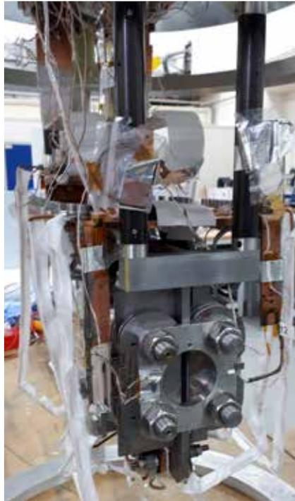
The superconducting undulator prototype before insertion into the cryostat.
