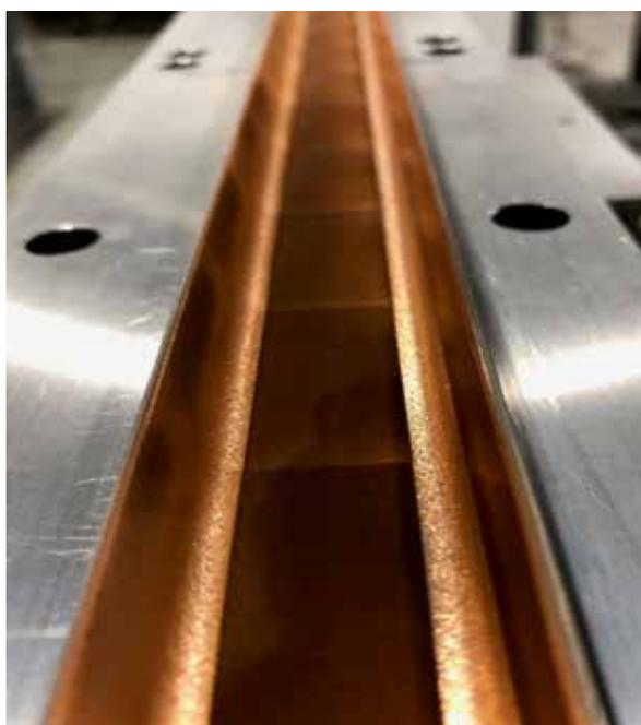
The FCC vacuum chamber prototypes after LASE treatment
